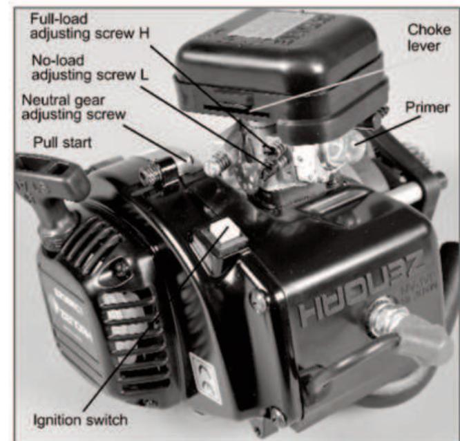
During the first two tank fillings, avoid running at maximum speed ranges in no-load condition as well as full-speed drives on long straight lines. It is advised to check the effective range of the radio control system with the engine running.
